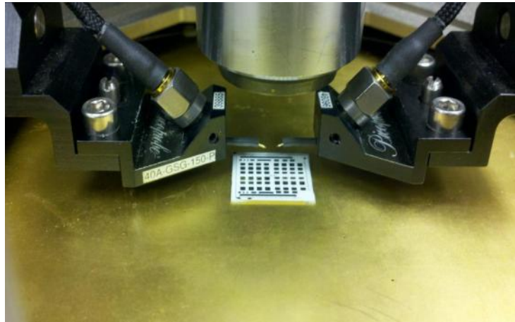
Figure 6-2: Alumina Sample on Temperature Controlled Chuck
